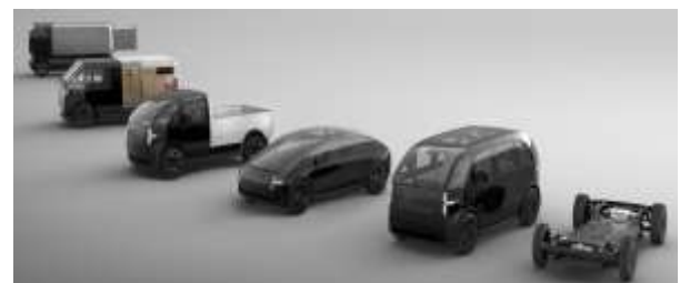
Fig. 3. EV configurations in Canoo's "skateboard" design
