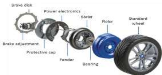
Fig. 11. Electric motor is integrated into the wheel
