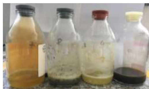
Fig. 4. After digestion of oyster tissue with different agents (From left to right: (a) HNO 3 ; (b) H 2 O 2 ; (c) mixture of Trypsin e and H 2 O 2 ; (d) NaOH)
