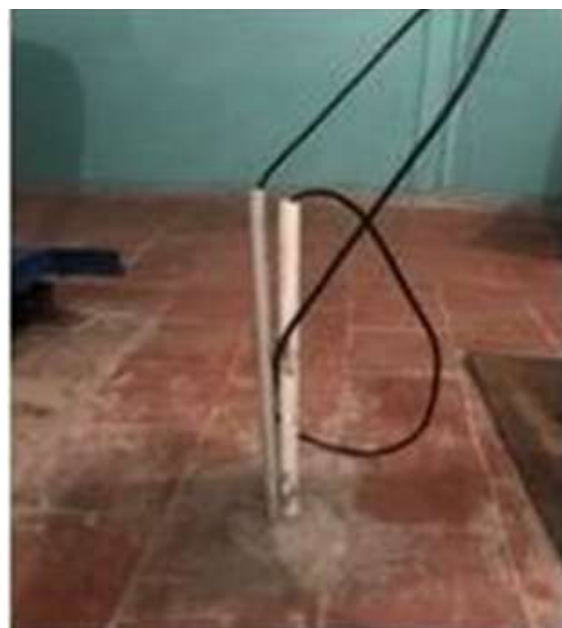
Figure 5. A pressure sensor for measuring soil pressure (taken from the open sources)
